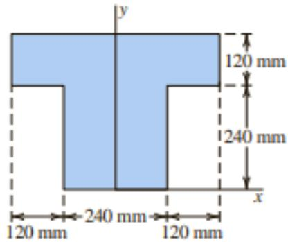
h) Determine the moments of inertia about x-axis and y-axis for the T-shaped area shown below.
